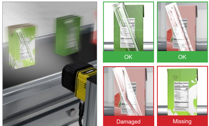
Food & beverage: Identify damaged or missing components
