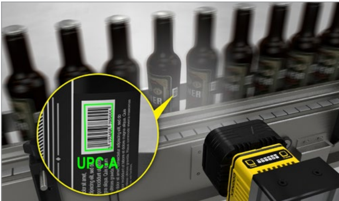
Barcode reading: Read codes on curved surfaces
